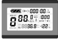
In the riding condition, 5 seconds later, a single maximum speed (MXS) display automatically returns to the real riding speed (Km/H).
