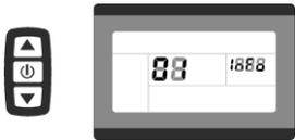
Electronic control system failure will display (flashing) fault code. Once the fault was removed, it automatically exits from the fault code display interface.
