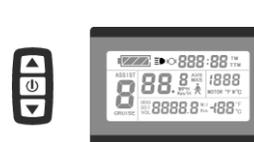
Hold long to turn on backlight and headlights (the controller should have headlight drive output function); hold long again to turn off the backlight and headlights.
